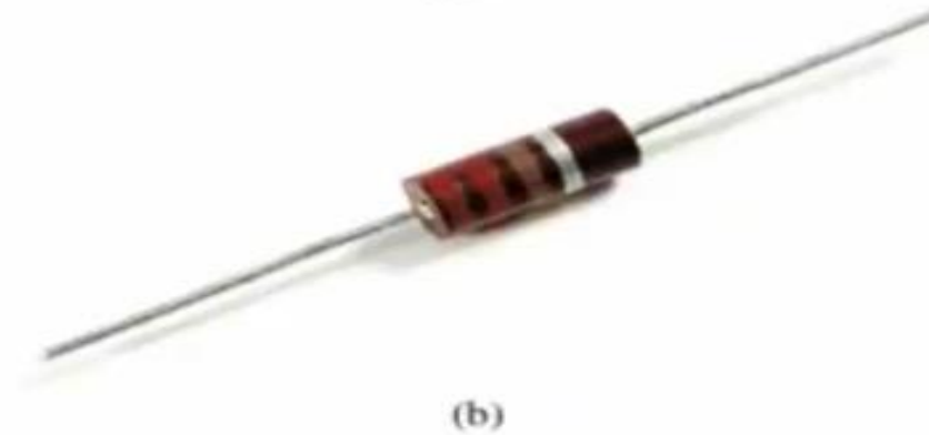
Fig3.5 : Fixed-composition resistors: (a) construction; (b) appearance
