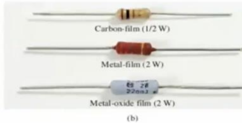
Fig3.4 Film resistors: (a) construction; (b) types.
